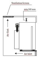
Please note that the minibar must be properly ventilated, otherwise minibar will not work efficiently. The diagrams illustrate the perfects ways of installing a minibar. Air inlet and outlet openings (each) must be at least 200 cm<sup>2</sup>. If you don't have adequate ventillation for your minibar, minibar might give faulty results.
